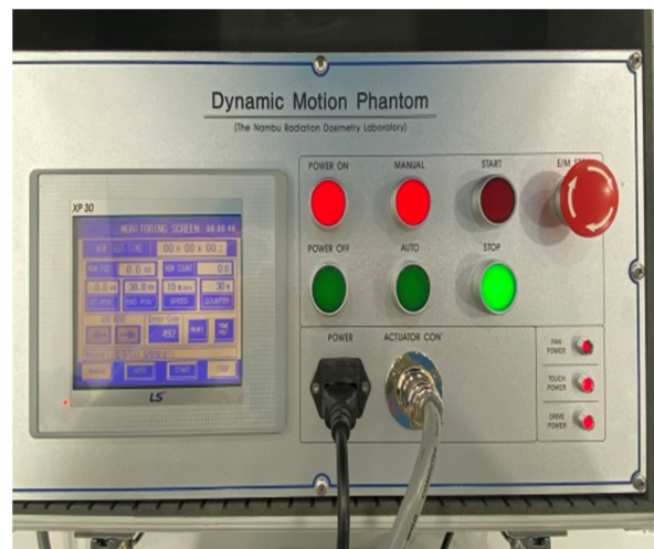
Figure 3. Position and speed control module
